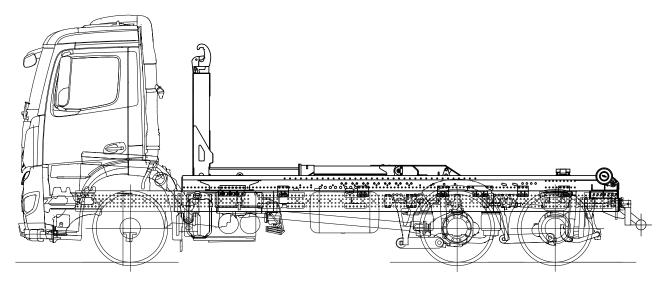
The chassis with the mounted **HOOKLIFT S-20** model hook-lift equipped container transporter superstructure is a target machine that can load behind the vehicle and unload by tilting. It's useful lifting capacity is 20,000 kg. With containers that are designed for specific purposes and comply with the DIN 30722 standard it can be used:
